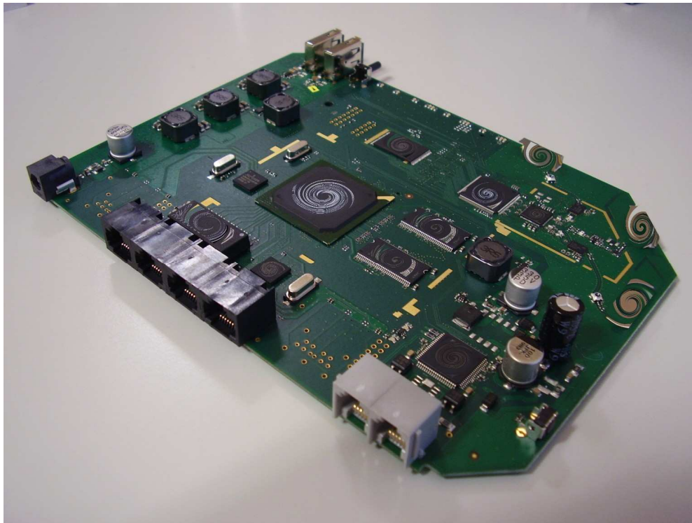
Figure 3.11 – ALPHA Residential Gateway board provided by Telsey
