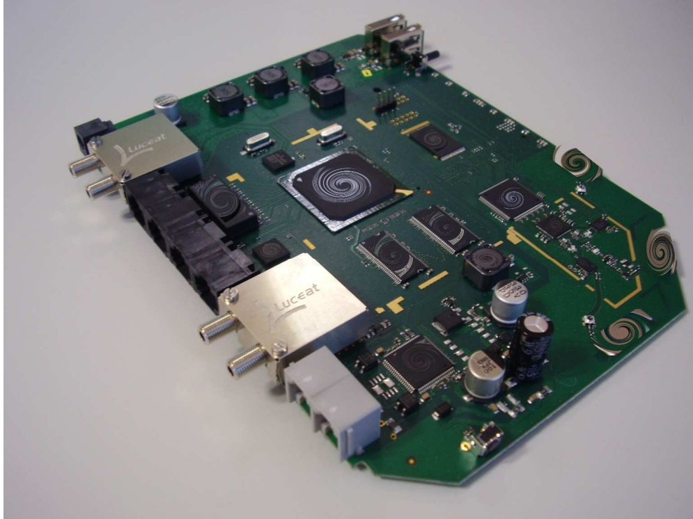
Figure 3.12 – ALPHA Residential Gateway board (1)
